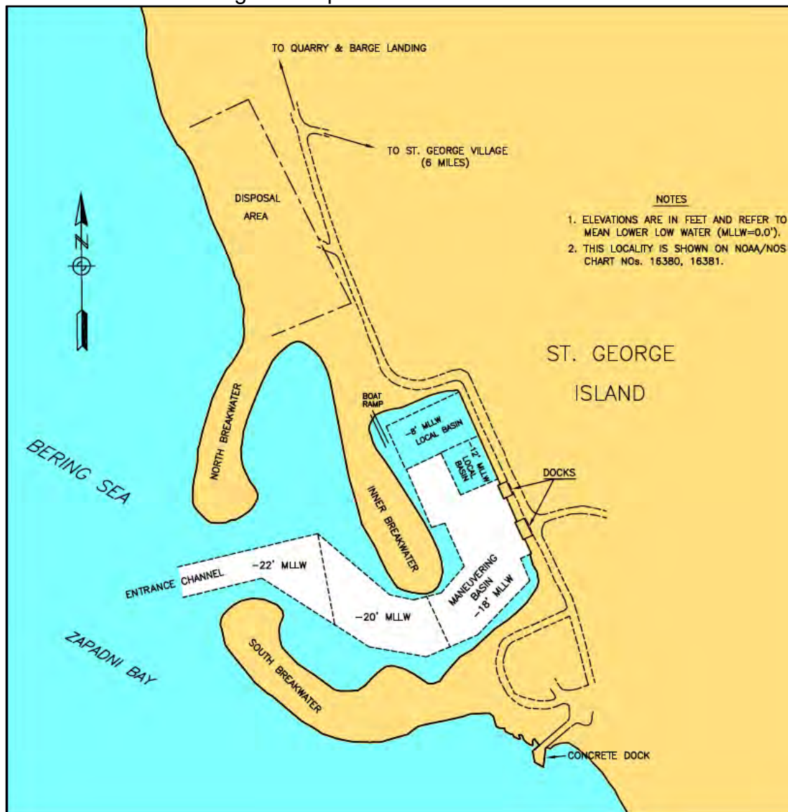
Figure 7. St. George Harbor Federally-maintained Portion in White (suspended). The locally-maintained portion is in blue.
