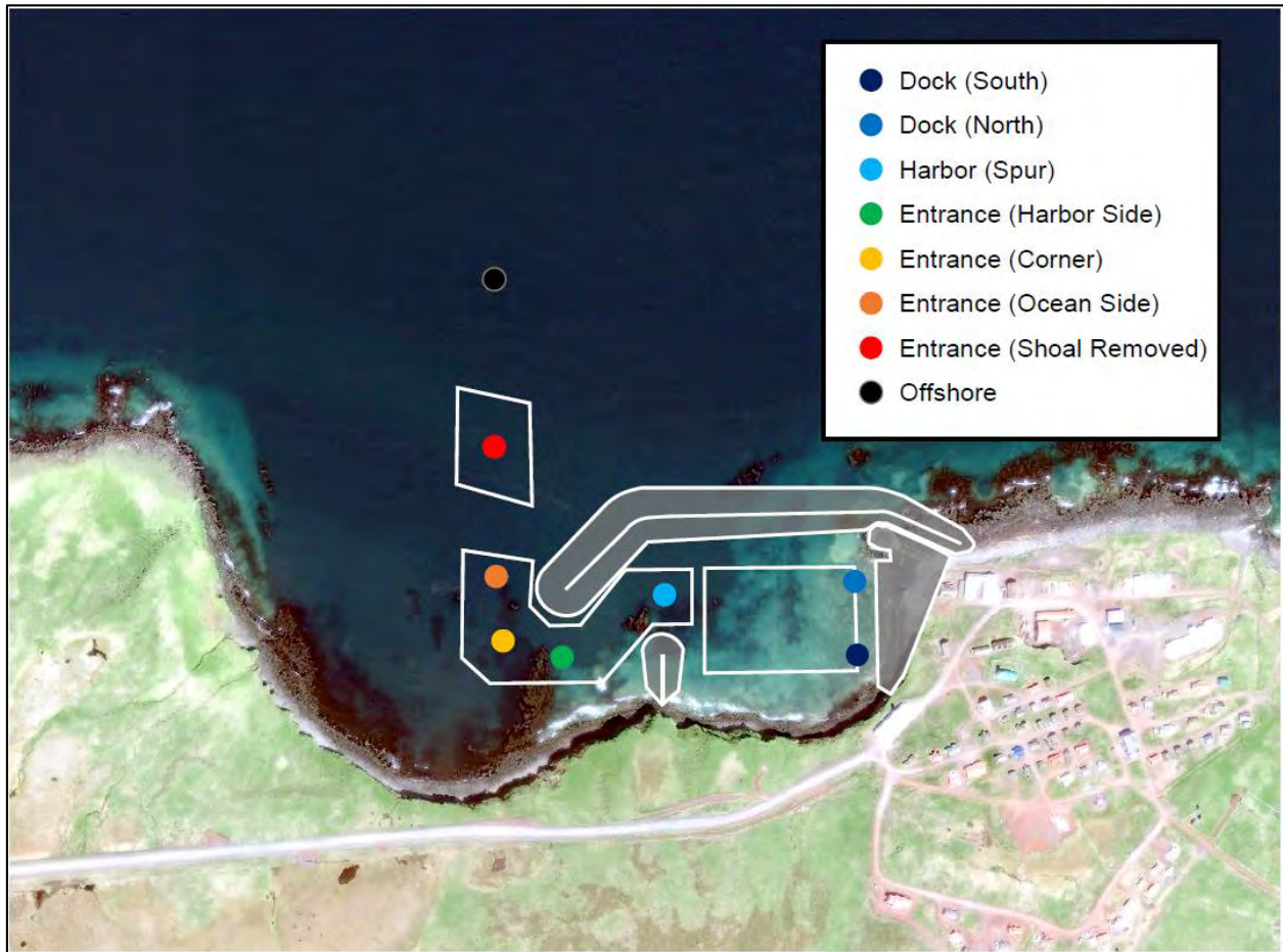
Figure 62. Output locations for the BOUSS2D Model.
